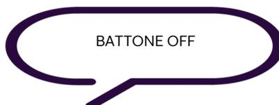
To reactivate dial tone (battery alarm/low battery voltage indication, dial tone) send the below SMS to the LTE Gateway. The Gateway will return an acknowledgement:
