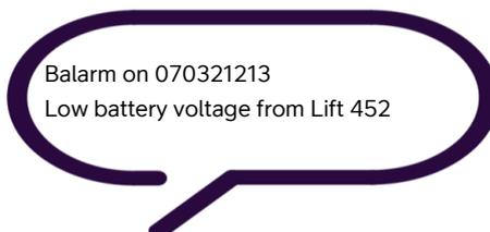
In this example a Low battery voltage indication will generate the following:
