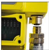
For mounting the sensor must be plugged into the socket and screwed on the sensor by turning the lower knurled screw clockwise. Tighten hand-screwed only.
