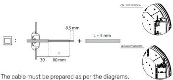
The conductors must be stripped for a length of 8.5mm. Respect the polarity.
